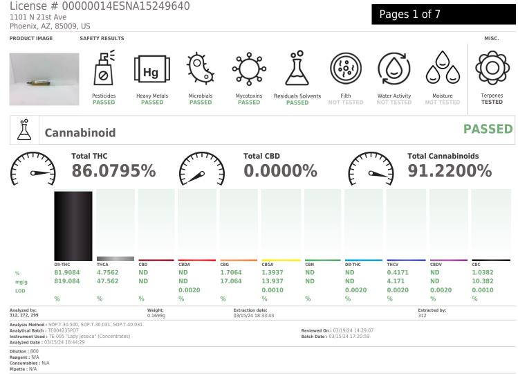
Full spectrum cannabinoid analysis utilizing High Performance Liquid Chromatography with Photo Diode Array detector (HPLC-PDA) for analysis. (Methods: SOP.T.30.500 for sample homogenization, SOP.T.30.031 for sample prep, SOP.T.40.031 for analysis on Shimadzu LC-20X0 series HPLCs). Potency results for cannabis flower products are reported on an "as received" basis, without moisture correction.
